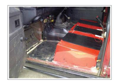
Now to install the seat box cover, you will need to lay the carpet panels on the seat box and line up the positions on the seat box with the correct cut outs on the panels. Bond the panels into place to achieve the best result. You will need to remove or cut around the under seat storage plate fixings, handbrake and replace them back once the carpet has been fitted.
